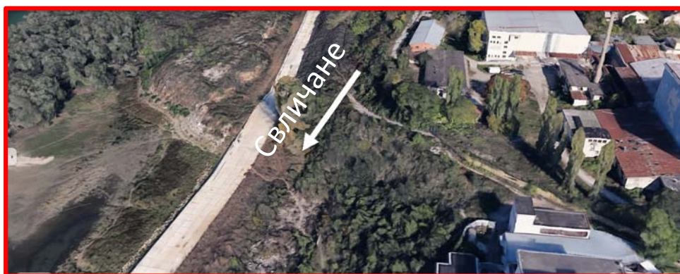
Fig. 5. Second example - Subsidence of the earth layers, found in an industrial zone in the city of Ruse. There is a dangerous tendency for the subsidence to turn into a landslide.
